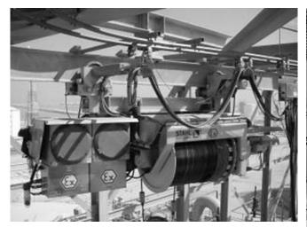
With safe working loads between 63 and 6,300 kg, explosion-protected versions, modular design and countless off-standard solutions, STAHL CraneSystems hoists are equipped for the most varied applications.
